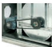
Motor outside the airflow path
